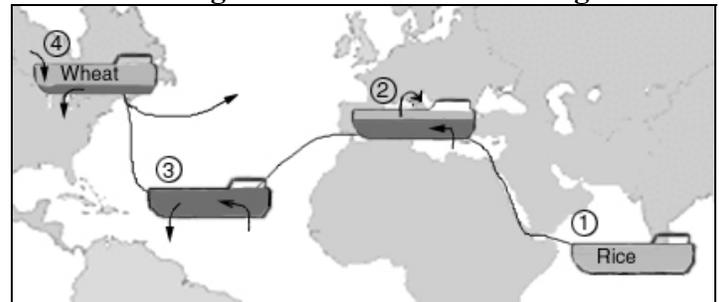
Figure 1 illustrates how ballast water exchange would work. A ship leaves a port in the Indian Ocean, travels through the Suez Canal, discharges cargo in the Mediterranean and takes up ballast water prior to crossing the Atlantic Ocean. Ballast water exchange would occur in the Atlantic prior to the ship entering the Great Lakes to pick up cargo, e.g. wheat for transport to the receiving port.
