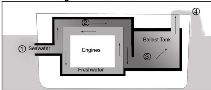
1. Sea water is pumped in to flush ballast tanks. 2. The sea water is heated (shown in a darker shade) by freshwater used to cool the ship's engines. 3. The heated sea water is pumped into the ballast tanks, killing many of the organisms. 4. The treated ballast water is pumped overboard.
