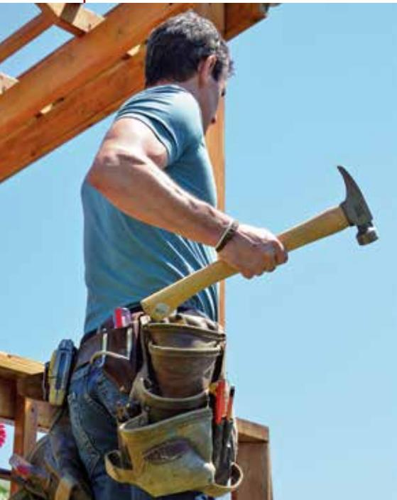
Do deck builders really need axe-handle hammers? After all, we're not framing walls, where a curved handle would enable us to swing around the end of the plate more efficiently. And even if we were, chances are good that we'd be using a nail gun instead of a hammer. But it turns out that even for a deck builder, Stiletto's 12-ounce, 18-inch framer's hammer is pretty handy.
