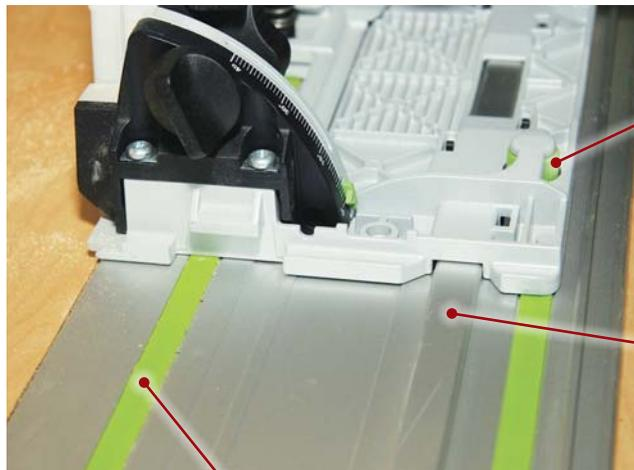
Two adjustable cams allow the fit to be fine-tuned.
