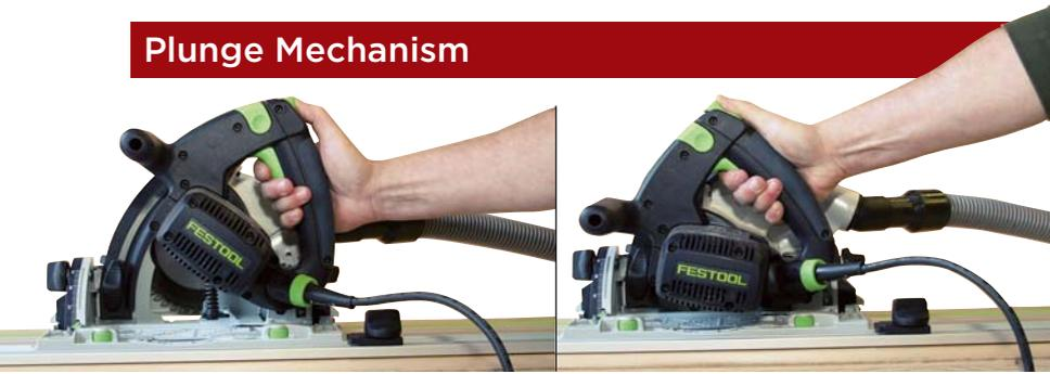
The plunge mechanisms on the Festool and Makita are similar: The operator presses a plunge release with his thumb, then pivots the motor down until it bottoms out against the depth stop. It's easy to do one-handed, with a forward twist of the wrist.
