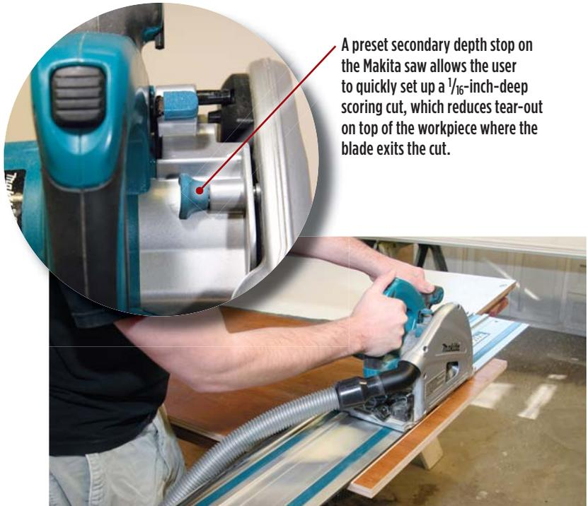
A preset secondary depth stop on the Makita saw allows the user to quickly set up a  $\frac{1}{16}$ -inch-deep scoring cut, which reduces tear-out on top of the workpiece where the blade exits the cut.
