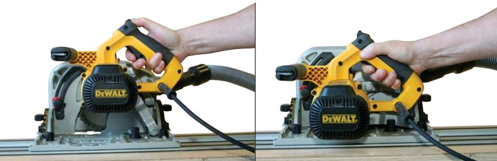
The DeWalt's motor is connected to the base by a pair of parallel plates, so it pivots forward and down without changing the orientation of the grip. The action is more comfortable than plunging the Festool or Makita, but it's harder to do one-handed.
