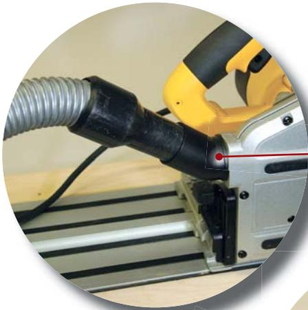
When connected to a vacuum, plunge-cutting saws do an excellent job of collecting dust. Any vac will do, as long as it's powerful. The hose connects to a rotating port on the back of the blade housing.
